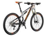
Material: Hydroformed and custom butted 6061 aluminium Fork: Rockshox FOX 34 Float Performance Air | 150 mm Rear Shock: FOX Nude | SCOTT Brakes: Shimano SLX M675 Disc | 180/180 mm
