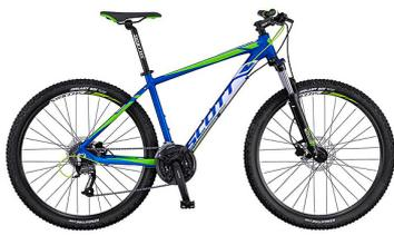
**Rahmen:** Aspect 700 series Alloy 6061 Performance geometry Internal cable routing
